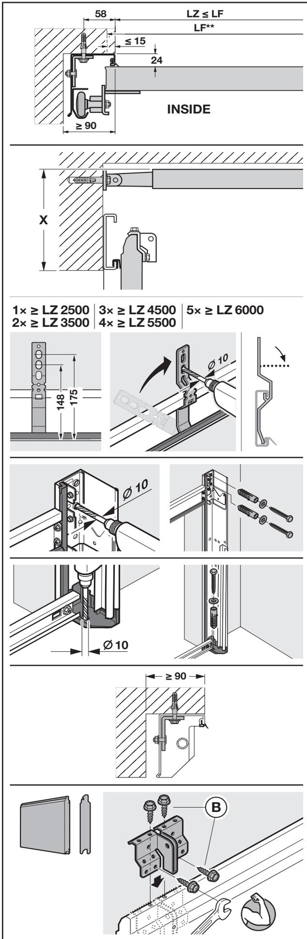
Frame legs must be fitted behind the reveals with a centreline for the fittings at 58mm from the edge of the structure.
