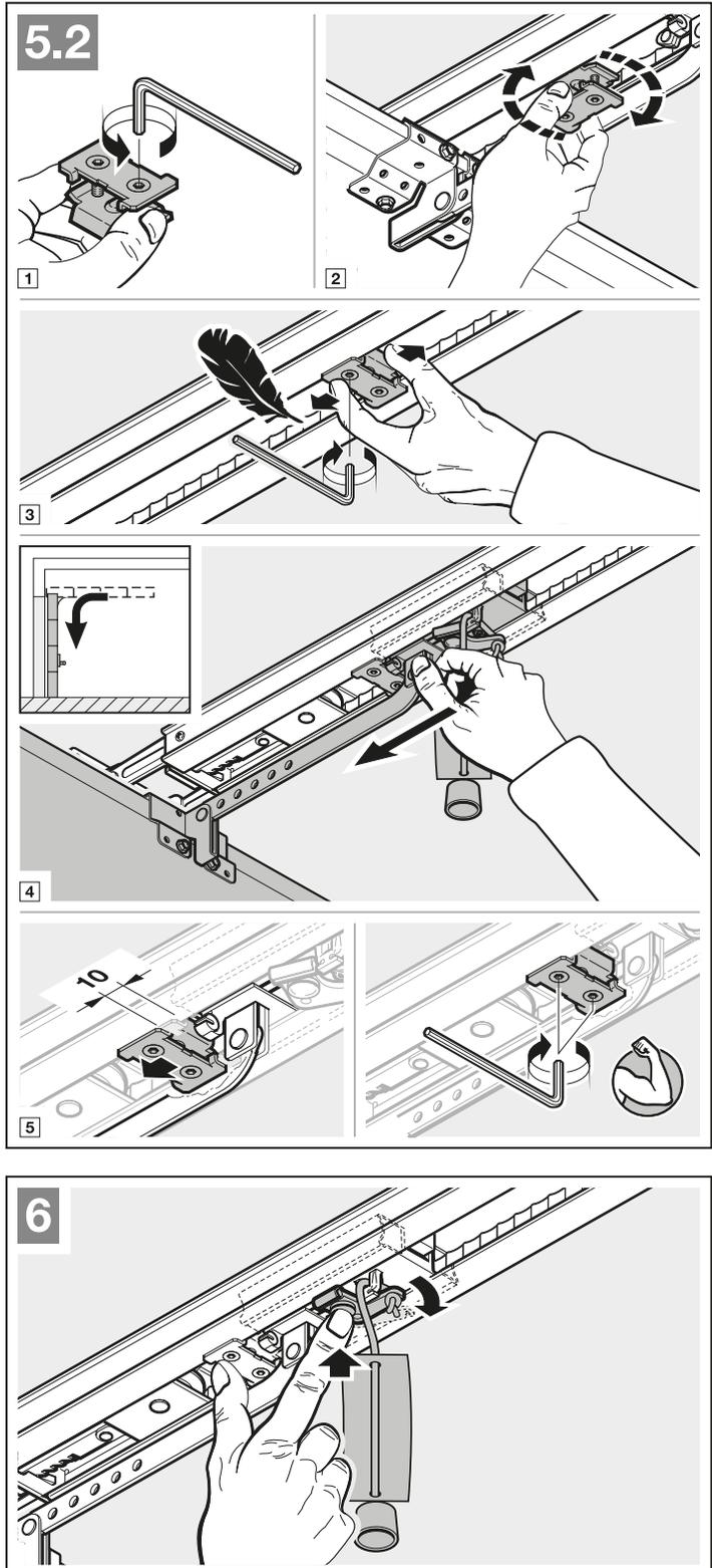
**3.5.3 Fitting the operator head**
