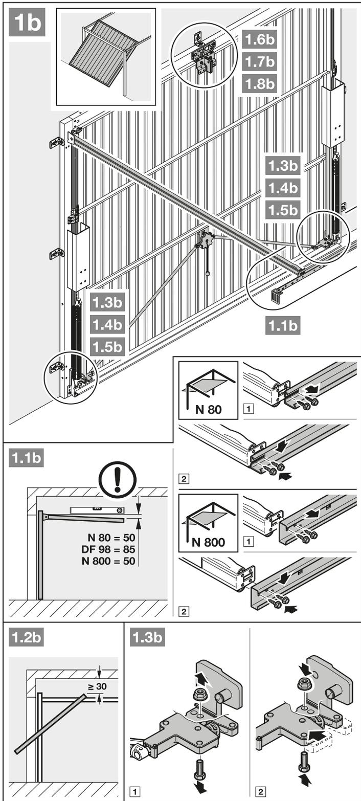
2. Render the mechanical door lockings inoperable (see Figures 1.4b / 1.5b). For door models not covered here, block the catches on site.
